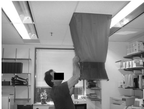
Fig. 3. Device for measuring airflow volume.
