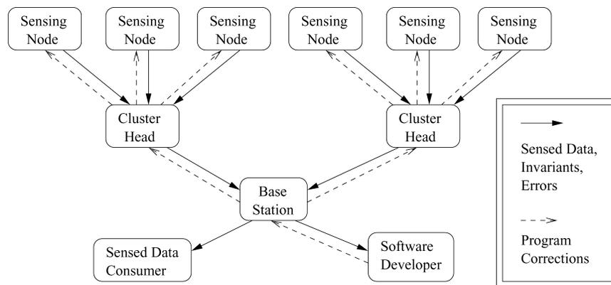
Fig. 2. Overview of the framework for fault detection, propagation, diagnosis, and repair.
